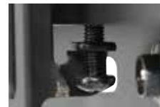
Securing screws lock adaptor to wall plate
