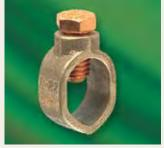
This heavy duty ground rod clamp replaces all existing ground rod clamps, eliminating the need to stock several different sizes and types. UL listed for direct burial in earth and concrete, the heavy duty construction enables it to handle large ground wires up to 1/0 AWG – much larger than a standard ground rod clamp. Suitable for: \%", \%", \%", \%" ground rods.
