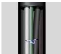
Parallel Arc Fault
