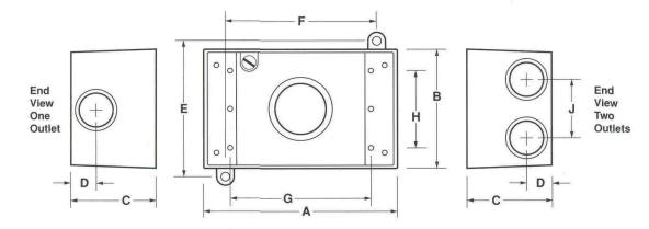
Extensions and Extension Adapters are used to provide additional capacity needed for NEC box fill requirements. Adapters allow installer to add "take-offs" to new boxes and/or devices.
